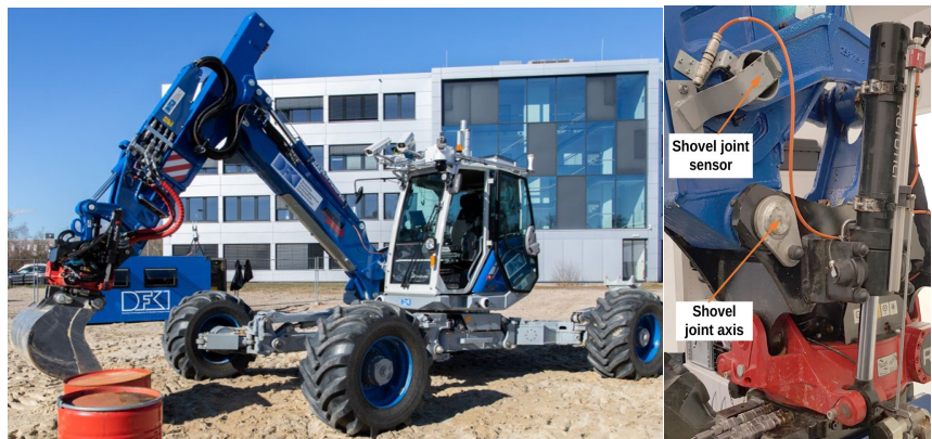
Figure 8. ARTER robot (left) and the robot's Shovel joint (right).
