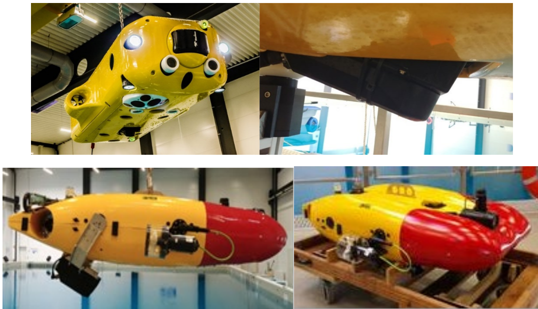
Figure 5 The AUVs Flatfish (top) and Dagon (bottom) equipped with the Gemini 720i FLS.
