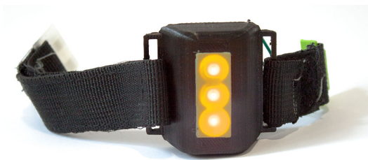
Figure 1: The notification device which is worn on the wrist. It is powered by an RFDuino equipped with three RGB LEDs and a vibration motor.
