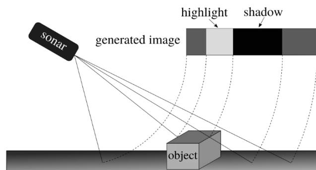
Figure 2.6: Example of a generated image using one beam
