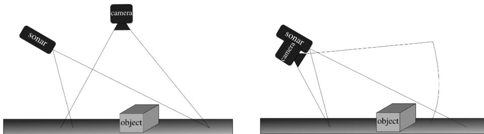
Figure 2.9: Schematic depicting possible positions of the imaging sonar and camera
