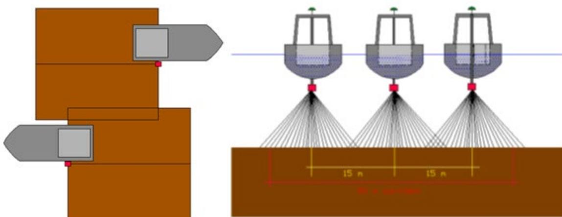
Figure 4.7.: Multibeam survey overlap example.
