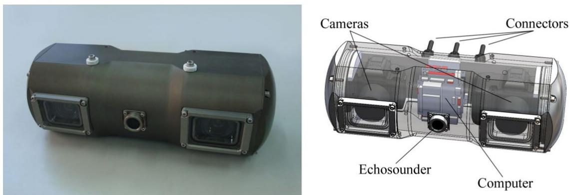
Figure 4.13: Camera Stereo schematic
