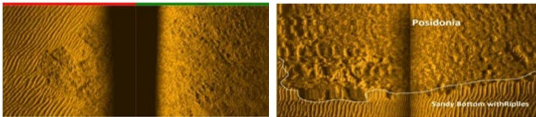
Figure 4.3: Left, side scan sonar record of cemented sands. Right, Posidonia field and sandy bottom with ripples.
