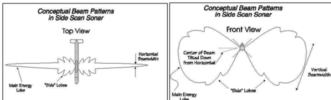
Figure 4.1: Beam patterns scheme of an SSS.
