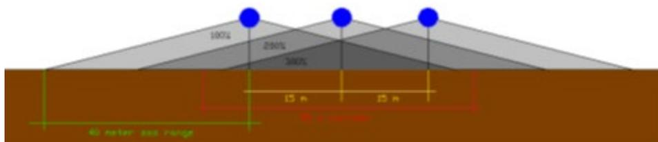
Figure 4.2: Side scan sonar survey overlap example.
