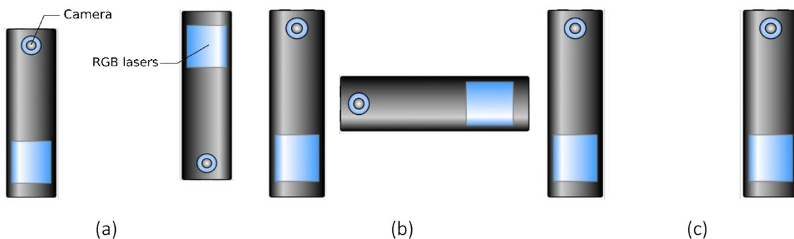
Figure 2.3: Possible SeaVision Twin mounting configuration
