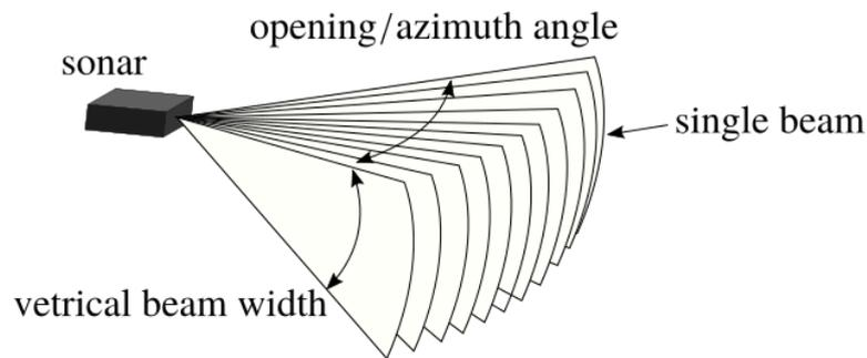
Figure 2.5: Schematic showing the acoustic beams emitted by a multibeam sonar
