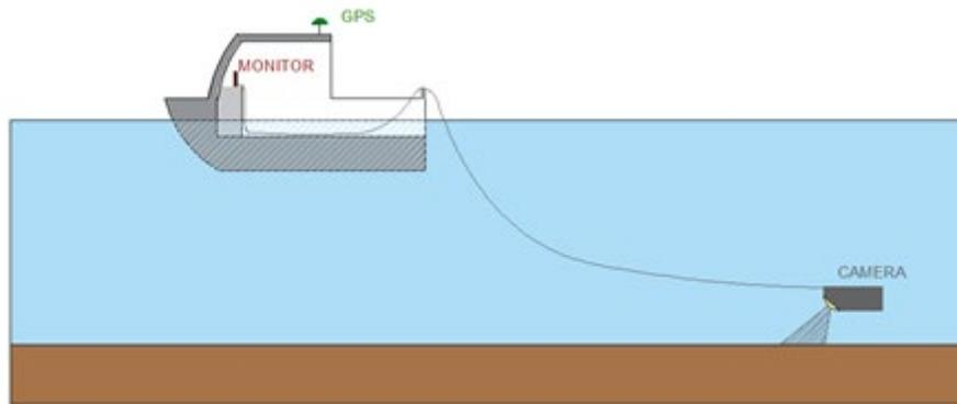
Figure 4.9: Towed camera deployment.
